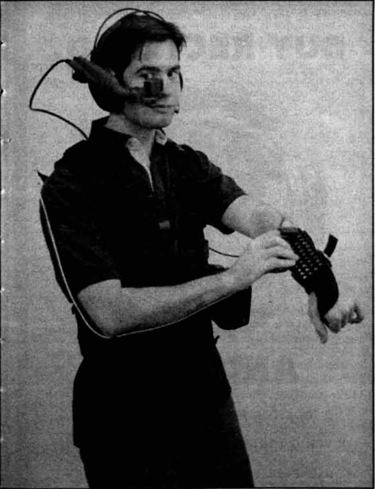
David T. Pinson '01 ports his team's wearable computer intended to serve as a biomonitoring tool for astronauts. He and fellow team members will test the device on the KC-135A reduced gravity aircraft this Saturday.
