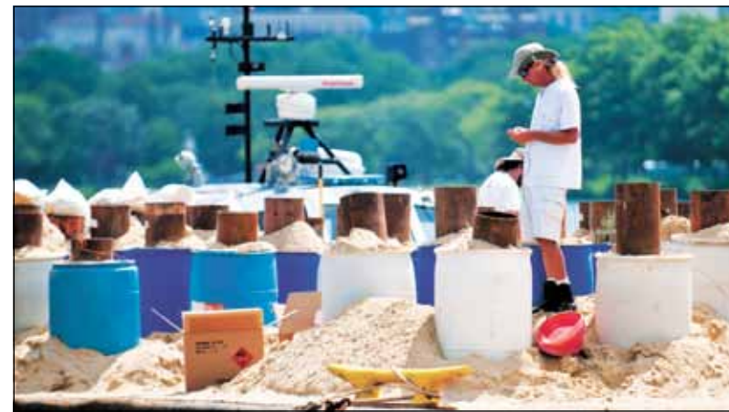
A worker makes electrical connections to a fireworks shell that has been loaded into its firing tube midday Saturday.
