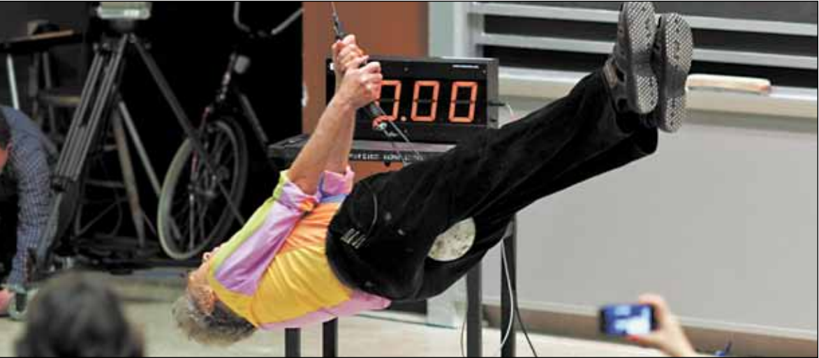
MANOHAR SRIKANTH—THE TECH The 75-year-old Professor Lewin takes 10 full swings on a pendulum to demonstrate that adding mass will not change its frequency.
