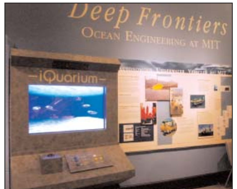
The iQuarium, one of the four iCampus projects to receive funding this year, is located in the Hart Nautical Gallery on the ground floor of Building 5. The iQuarium is a computerized virtual aquarium, employing a trackball that allows the user to pan through a virtual fish tank and see the vortices created in the wakes of passing fish. BRIAN HEMOND—THE TECH
